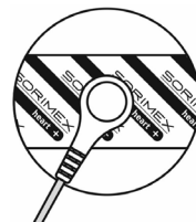
Fig. 1. Way of leadwire and electrode connection
